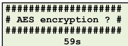
In order to enable the encryption, user shall set the key in the horizontal position and keep the OK key pressed for approx. 10 seconds. The recorder will notify the user about the encryption setup.
