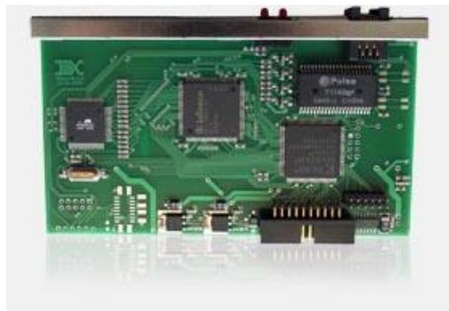
ISDN 30B+D digital trunk adapter (PRA, E1, G703 protocol, DSS1 or MFC R2 signaling). The full board consists of 30 voice channels and two data channels (control). This adapter connects the recorder directly to the digital PABX.
