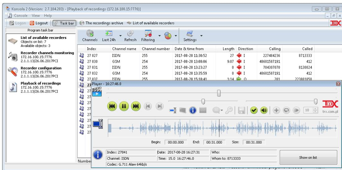
The main operating program is “Konsola 2.” Its friendly user interface gives access to all (allowed by the user’s security level) recorder’s functions. It allows playback, channel monitoring, and archiving without interruption in recorder’s work. It lets configure the system in the deepest detail. It also has plenty of convenient features, like searching (sorting) the calls by age, by channel, by telephone number, by comment or *even* by call duration.
