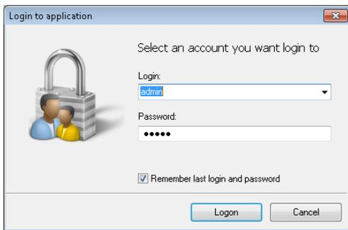
The users are authorized in the system in a username/password routine. The authorization system can also be integrated to Windows™ operating system or Radius® identification system (if the computer has Radius® protocol chip-card reader installed).
