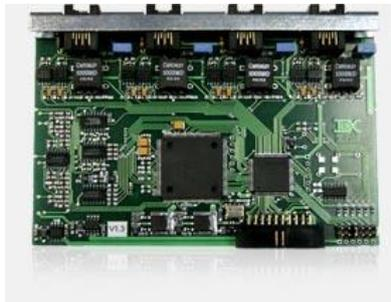
Analog line adapter supports analog signal sources such as telephone line, radiotelephone or microphone. DSP allows the analysis of incoming and outgoing calls numbers.
