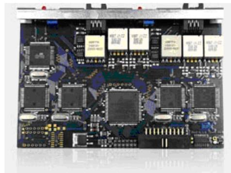
2B+D (BRA, S0) ISDN line adapter. Each socket supports two voice channels. Two versions are available:
