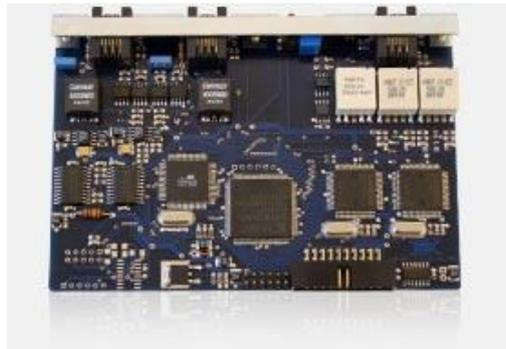
You can connect two analog phone lines and one ISDN line, which means that the card is able to record from two channels of analog and two channels of an ISDN line talkative. For ISDN channels analysis is numbers.
