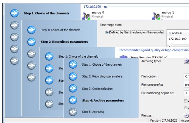
The data is archived on a remote computer where it is transferred over LAN/WAN network. The archive size can be freely modified (the maximum size, due to Windows file system limitation is 2 GB) and adjusted to fit the CD-R or DVD-R drive.
