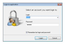
The users are authorized in the system in a username/password routine. The authorization system can also be integrated to Windows<sup>TM</sup> operating system or Radius<sup>®</sup> identification system (if the computer has Radius® protocol chip-card reader installed).
