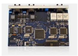
You can connect two analog phone lines and one ISDN line, which means that the card is able to record from two channels of analog and two channels of an ISDN line talkative. For ISDN channels analysis is numbers.
