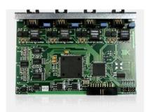
Analog line adapter supports analog signal sources such as telephone line, radiotelephone or microphone. DSP allows the analysis of incoming and outgoing calls numbers.
