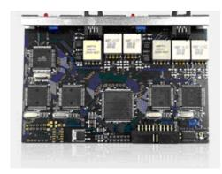
2B+D (BRA, S0) ISDN line adapter. Each socket supports two voice channels. Two versions are available:
